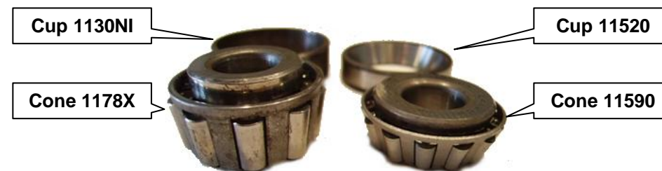
Origineel (OLD) en vervangend lager (NEW)
